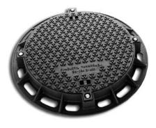
**Sealed cover and frame** bearing a pressure of up to 1 bar. **Sealed closure** (both sides) with four stainless steel screws and special elastomeric gasket.
