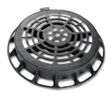
Locking is made by means of three flaps at the bottom of the cover, making a twist of 5 cm, the cover remaining combined (as if it would be screwed); the third flap has integrated an iron lock with threaded holes, which remains blocked.
